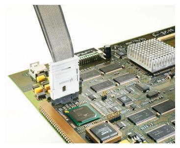
E5346A 34-channel Mictor connector probe
