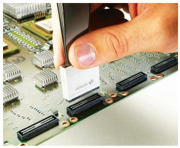
E5385A 34-channel Samtec connector probe
