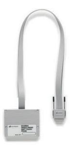
E5396A 16-channel soft touch connectorless probe
