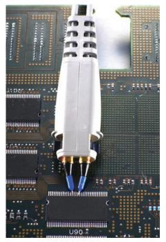
InfiniiMax solder-in probe head with long wires
