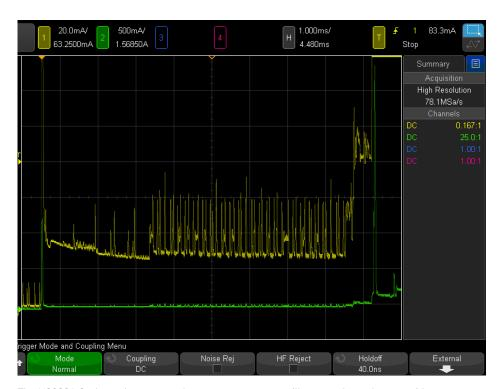
The N2820A 2-channel current probe connects to two oscilloscope channels to provide simultaneous low- and high-gain views for wider dynamic range measurement
