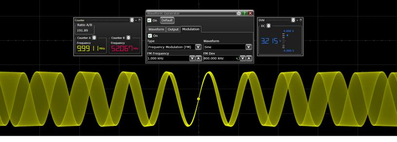
Generating a 10 MHz sine wave with frequency modulation, while measuring two signal frequencies with counters and a third signal's DC voltage with the DVM. Note that channels need not be enabled for the counter and DVM to operate.
