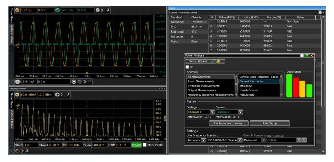
This application enables a broad range of automated power supply characterization measurements from input analysis, switching device characterization, and output analysis. It also includes critical frequency response measurements such as power supply rejection ratio (PSRR) and control loop response.
